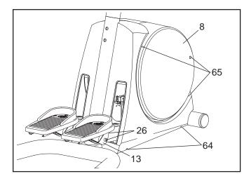
Remove the right Pedal Bracket (13) by removing the two M10 x 82mm Button Bolts (26) and the two M10 Nylon Locknuts (not shown). Then, remove the two M4 x 38mm Screws (64) and the three M4 x 25mm Screws (65). Carefully slide the Right Side Shield (8) off the stepper.
